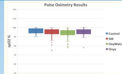
**Figure 1:** Illustrates the findings of a study that examined pulse oximetry readings by the following devices Santa, Medical SM-165 (SM), Walgreens' OxyWatch C20 (OxyWatch), and Nonin Onyx II 9550 (Onyx). Each data point represents the oxygen reading for one patient. 50.5% of the patient population was African American in this study. The oxygen percentage data shown includes outliers and mean lines.<sup>2</sup>
