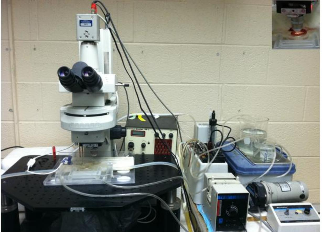
Figure 5: Experimental setup for intravital microscopy. Inserted picture in upper right → Exteriorized loop of mesenteric tissue undergoing superfusion of test solution.
